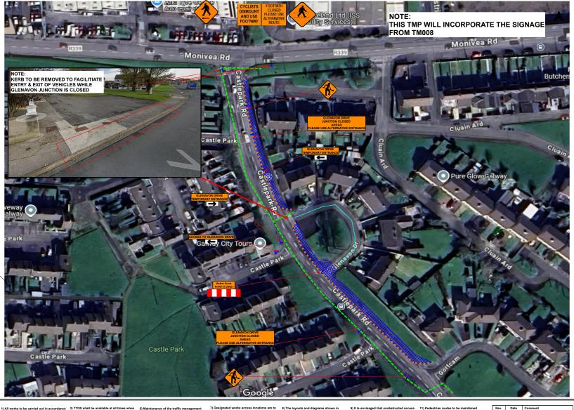
ROAD / WORKS CHARACTERISTICS Speed Limit Roadworks Type (50) 1(iii) Α Single or Multi-Lane / Dual Sign Size Single 600mm TEMPORARY SIGNS Sign Visibility Number of Signs Sign Spacing 50m 2 20m MIN. RATE OF TAPER Taper at Lane Taper At Transition Hard Shoulder Length 1 in 5 1 in 5 SAFETY ZONES & LANE WIDTH Longitudinal Safety Zone Minimum Lateral Lane Width 0.5m 3m CONE SIZE & SPAC Minimum Cone Height Spacing at Tapers Longitudinal Spacing 750mm 3m 3m Lamp Spacing Longitudinal Lamp Spacing 6m 6m
